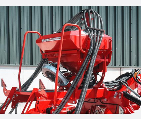
Fitted with an Accord pneumatic distribution system, it is suitable for sowing oilseed rape, grass, cover crops, slug pellets and a wide range of seeds up to 12 metre working width.
