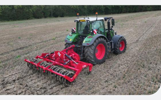
The ultra-low disturbance heaving action of the LD Top-Soiler relieves compaction in the top 9" (228mm) of the root zone, providing soil aeration and better water infiltration, while leaving the soil surface virtually undisturbed. The legs are followed by a heavy duty cast ring roller which leaves an even surface finish.
