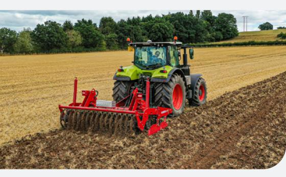
The low draft legs are designed to break up the soil pan and aerating the soil without creating much disturbance to the soil surface, whilst the discs are able to chop and mix crop residues and create a stale seedbed, with the packer roller leaving a level finish.
