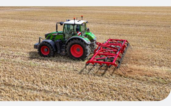
With its unique tine configuration and design, the Weaving Stubble Rake is able to create ideal conditions in which weed-seeds and volunteers will readily germinate allowing for control before drilling. This machine is able to decimate slug eggs and weeds including black grass in growing crops. The Stubble Rake is used at high speeds and is able to work over a large acreage in a short amount of time.
