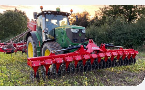
With front linkage mounting and a full width set of wavy discs, it is able to cut through trash and cover crops in front of the drill, clearing the path for the drill to both improve seed to soil contact and prevent debris from hooking around the coulters and causing blockages.
