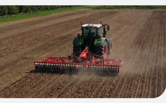
Working depth is between 0 and 15cm (6"). 167mm spacing between legs is similar to our Sabre drill allowing for high volumes of trash to flow through and ensure all ground is worked.
